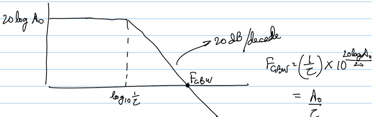
The loop gain of the above system which has to be considered to make the system stable is given as:
