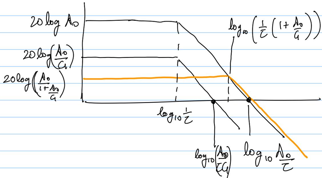
Although we have to work to stabilize with pole at  $\frac{1}{zeta}$  we get performance & bandwidth upto  $\frac{1}{zeta} \left( 1 + \frac{A_0}{a} \right) !!$
